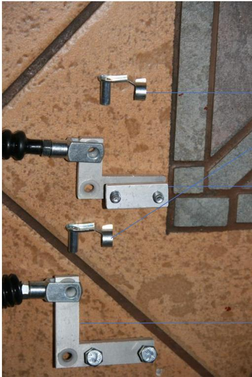
Clips removed from clevises (7) to enable change of clamps.
